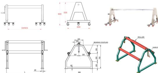
The Stationary Pool Roller is made from high grade, 316 stainless steel and is ideal for medium pools from 4m wide by 12m long to large pools upto 6.5m wide by 30m long.
