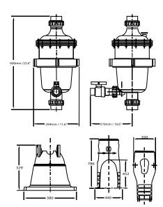
MultiCyclone is a centrifugal filtration device that is capable of saving water and reducing filter maintenance.
