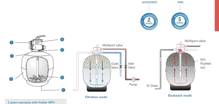
High performance top mounted sand filters are manufactured with polyester and glass fiber winding for dependable, durable and all weather operation.
